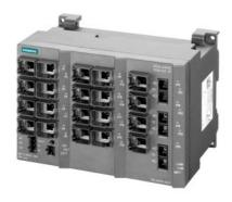
SCALANCE X320-3LDFE managed IE switch, 20x 10/100 Mbit/s RJ45 ports, 1x 100 Mbit/s SC Port MM 2x 100 Mbit/s SC Port SM LED diagnostics, error signaling contact with select/set pushbutton, PROFINET IO device, network management, integrated redundancy manager, office features (RSTP, VLAN, IGMP,...) C-PLUG in scope of supply.
