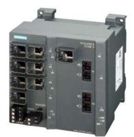
SCALANCE X308-2, managed plus IE switch, 2x 1000 Mbit/s MM SC 1x 10/100/1000 Mbit/s and 7x 10/100 Mbit/s RJ45 ports, LED diagnostics, error signaling contact with select/set pushbutton, PROFINET IO device, network management, integrated redundancy manager, office features (RSTP, VLAN, IGMP,..) C-PLUG in scope of supply.
