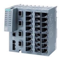
SCALANCE XC224-4C G manageable Layer 2 IE switch; IEC 62443-4-2 certified; Full gigabit; 20x 10/100/1000 Mbps RJ45 ports; 4x 1000 Mbps combo ports (either 1000 Mbps/ SFPs or 10/100/1000 Mbps RJ45 ports can be used); 1x console port; diagnostics LED; redundant power supply; temperature range -40 °C to +70 °C; assembly: DlN rail/S7 mounting rail/wall; redundancy functions; office features (RSTP, VLAN,...); PROFINET IO device; Ethernet/IP-compliant; C-PLUG slot; IEEE 1588v2 PTP
