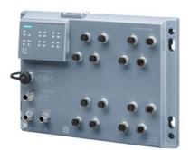
SCALANCE XP216EEC, managed IE switch, with railway approval IEC 62443-4-2 certified; (EN 50155, EN45545); 12x 10/100 Mbit/s M12 ports, 4x 10/100/1000 Mbit/s M12 ports IP65, LED diagnostics, error signaling contact, redundant power supply, PROFINET IO device, network management, can be operated in redundant ring, incl. dust caps, including electronic manual on CD-ROM, C-PLUG optional.
