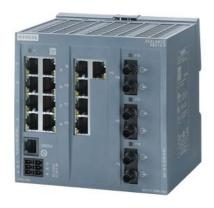
SCALANCE XB213-3 managed Layer 2 IE switch 13x 10/100 Mbit/s RJ45 ports, 3x MM FO ST port 1x console port, diagnostics LED, redundant power supply, IEC 62443-4-2 certified; temperature range 0 °C to +60 °C; DIN-rail mounting; default EtherNet/IP.
