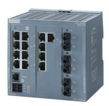
SCALANCE XB213-3 managed Layer 2 IE switch 13x 10/100 Mbit/s RJ45 ports, 3x MM FO ST port 1x console port, diagnostics LED, redundant power supply, IEC 62443-4-2 certified; temperature range 0 °C to +60 °C; DIN-rail mounting; default PROFINET.
