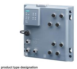
SCALANCE XP208PoE EEC, managed IE switch, 8x 10/100 Mbit/s IEC 62443-4-2 certified; M12 ports, IP65, LED diagnostics, error signaling contact, redundant power supply, PROFINET IO device, network management, can be operated in redundant ring, dust caps, including electronic manual on CD-ROM, C-plug optional.
