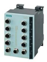
SCALANCE X208PRO, managed IE switch, 8x 10/100 Mbit/s M12 ports, IP65/67, LED diagnostics, error signaling contact, Redundant power supply, PROFINET IO device, network management, can be operated in redundant ring, dust caps, including electronic manual on CD-ROM, C-plug optional.
