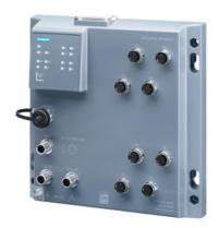
SCALANCE XP208EEC, managed IE switch with railway approval IEC 62443-4-2 certified; (EN 50155, EN 45545); 8x 10/100 Mbit/s M12 ports, IP65, LED diagnostics, error signaling contact, redundant power supply, PROFINET IO device, network management, can be operated in redundant ring, dust caps, including electronic manual on CD-ROM, C-plug optional.
