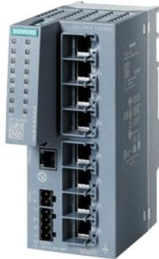
SCALANCE XC208EEC manageable Layer 2 IE switch; IEC 62443-4-2 certified; 8x 10/100 Mbit/s RJ45 ports; 1x console port; diagnostics LED; redundant power supply; with painted printed-circuit boards; NAMUR NE21-compliant; temperature range -40 °C to +70 °C; assembly: DIN rail/S7 mounting rail/wall; redundancy functions; Office; features (RSTP, VLAN,...); PROFINET IO device; Ethernet/IP-compliant; C-PLUG slot;
