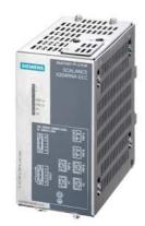
SCALANCE X204RNA EEC; redundant network access 2x 100 Mbit/s RJ45 ports; 2x 100 Mbit/s combo ports; LED diagnostics; error signaling contact with set pushbutton; simple power supply; network management; including electronic manual on CD-ROM, C-PLUG optional for PRP and HSR networks;.
