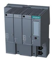
SCALANCE XF204 managed two BusAdapters BA 2xRJ45 HA IEC 62443-4-2 certified; IE switch, 4 x 10/100 Mbps, 2 x BusAdapter interface, error signaling contact, set pushbutton, redundant 24 V DC power supply, PROFINET device, extended temperature range -40 °C...+70 °C, conformal coating, with electronic manual on DVD, C-PLUG optional, delivery with BusAdapter. preassembled 6DL1193-6AR00-0AA0
