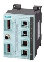
SCALANCE X202-2PIRT PRO, Managed IE IRT switch, Degree of protection IP65/67, 2x 10/100 Mbit/s Push Pull RJ45 ports, 2x 100 Mbit/s Push-pull SCRJ port; Error signaling contact with set pushbutton, Redundant power supply, PROFINET IO device; network management, Redundancy Manager integrated, incl. electron. manual on CD-ROM, C-plug optional.
