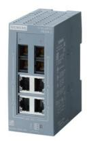
SCALANCE XB004-2 unmanaged Industrial Ethernet Switch for 10/100 Mbit/s; for setting up small star and line topologies; LED diagnostics, IP20, 24 V DC power supply, with 4x 10/100 Mbit/s twisted pair ports with RJ45 sockets; 2x 100 Mbit/s multimode glass fiber-optic cable port with SC socket; manual available as a download .
