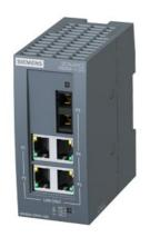
SCALANCE XB004-1LDG unmanaged Industrial Ethernet Switch for 10/100/1000 Mbit/s; for setting up small star and line topologies; LED diagnostics, IP20, 24 V DC power supply, with 4x 10/100/1000 Mbit/s RJ45 Ports electrical and 1 x 1000 Mbit/s SC-port optical (single-mode, glass), up to max. 10 km Manual available as a download .
