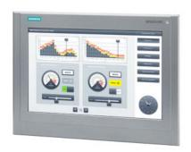
SIPLUS HMI TP1500 Comfort Outdoor based on 6AV2124-0QC13-0AX0 with conformal coating, -30...+60 °C, TP1500 Comfort Outdoor, Comfort Panel, touch operation, 15" widescreen TFT display, 16 million colors, PROFINET interface, MPI/PROFIBUS DP interface, 12 MB configuration memory, Windows CE 6.0, configurable WinCC Comfort V13 SP1 and higher, HSP
