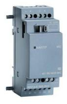
SIPLUS LOGO! AM2 based on 6ED1055-1MA00-0BA2 with conformal coating, -  $40...+70~^\circ\text{C}$  , start up -25  $^\circ\text{C}$  , expansion module, PS/: 12/24 V DC, 2 AI, 0-10 V or 0/4-20 mA for LOGO! 8
