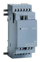
SIPLUS LOGO! DM8 24 based on 6ED1055-1CB00-0BA2 with conformal coating, -40...+70 °C, start up -25 °C, expansion module, power supply / I/O: 24 V/24 V/trans., 4 DI/4 DQ for LOGO! 8
