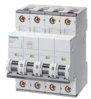
Miniature circuit breaker 400 V 10kA, 3+N-pole, D, 13 A, D=70 mm
