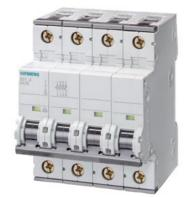
Miniature circuit breaker 400 V 10kA, 3+N-pole, C, 3 A, D=70 mm
