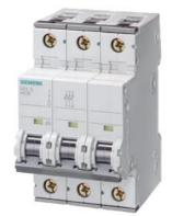
Miniature circuit breaker 400 V 10kA, 3-pole, D, 20 A, D=70 mm
