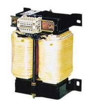
TRANSFORMER SITAS; PHASES:1; PN/PN(S6)(KVA):8 /28,5; UPRI(V):400+/-5%; USEC(V):230; ISEC(A):34,8; F(HZ):50...60; VECTOR GR./SHIELD WNG.:II0 /0; TA/ISOKL:55 /H; IP00; TYPE OF TERMINALS:SCREW CONNECTION; INSTALLATION:SCREW; EN 61558-2-1, -2-2, -2-4 >UL/CSA-RECOGNIZED< >CONTROL CIRCUIT TRANSFORMER< >ISOLATION TRANSFORMER<
