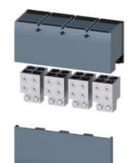
Wire connector TA4.4 4 x 4/0...600 kcmil for 4 cables; 4 units accessories for: 3VA55/3VA65/3VA66
