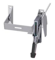
Operating Unit with Rod Variable Depth Flange Mounted operator kit, consisting of: handle steel epoxy coated NEMA 1, 12, 3R black=OFF, red=ON Switching mechanism Mounting depth 8" to 16" Accessory for: 3VA5 400, 3VA5 600 3VA6 400, 3VA6 600
