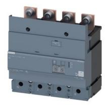
residual current device RCD820 advanced RCD type A load side mounted rated resid. current 0.03...30A at 50/60Hz adjustable tv 0...10000ms 4-pole In=630A Ue=100-690V accessory for: 3VA2
