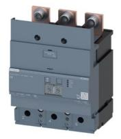
residual current device RCD820 advanced RCD type A load side mounted rated resid. current 0.03...30A at 50/60Hz adjustable tv 0...10000ms 3-pole In=630A Ue=100-690V accessory for: 3VA2
