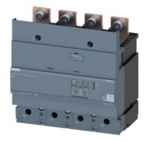
residual current device RCD820 advanced RCD type A load side mounted rated resid. current 0.03...30A at 50/60Hz adjustable tv 0...10000ms 4-pole In=400A Ue=100-690V accessory for: 3VA2
