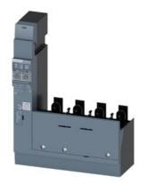
residual current device RCD510 Basic RCD type A side mounted rated resid. current 0.03...5A at 50/60Hz adjustable tv 0...3000ms 4-pole In=250A Ue=127-480V accessory for: 3VA1 with terminal connection
