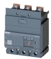
residual current device RCD520 Basic RCD type A load side mounted rated resid. current 0.03...5A at 50/60Hz adjustable tv 0...3000ms 3-pole In=250A Ue=100-480V accessory for: 3VA1
