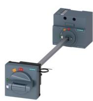
door mounted rotary operator standard NEMA type 1, 3R, 12, 4/4X with door interlock 24V DC lighting kit and door open position accessory for: 3VA4/5 125
