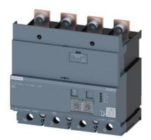
residual current device RCD820 advanced RCD type A load side mounted rated resid. current 0.03...30A at 50/60Hz adjustable tv 0...10000ms 4-pole In=160A Ue=100-690V accessory for: 3VA2
