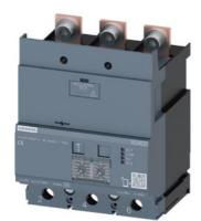
residual current device RCD820 advanced RCD type A load side mounted rated resid. current 0.03...30A at 50/60Hz adjustable tv 0...10000ms 3-pole In=160A Ue=100-690V accessory for: 3VA2
