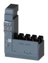
residual current device RCD510 Basic RCD type A side mounted rated resid. current 0.03...5A at 50/60Hz adjustable tv 0...3000ms 4-pole In=160A Ue=127-480V accessory for: 3VA1 with terminal connection
