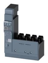
residual current device RCD310 Basic RCD type A side mounted rated resid. current 0.03...5A at 50/60Hz tv instantaneous 4-pole In=160A Ue=127-480V accessory for: 3VA1 with terminal connection
