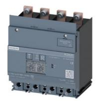
residual current device RCD520 Basic RCD type A load side mounted rated resid. current 0.03...5A at 50/60Hz adjustable tv 0...3000ms 4-pole In=160A Ue=100-480V accessory for: 3VA1
