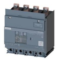
residual current device RCD320 Basic RCD type A load side mounted rated resid. current 0.03...5A at 50/60Hz tv instantaneous 4-pole In=160A Ue=100-480V
