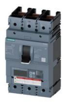
circuit breaker 3VA6 UL frame 600 breaking capacity class C 100kA @ 480V 3-pole, line protection ETU856, LSI, In=600A overload protection Ir=240A...600A short-circuit protection Isd=0.6..9x In, Ii=1.5..9x In N conductor protection optionally with external current transformer, up to 160% ground-fault alarm message via EFB300 or COM without connection
