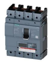
circuit breaker 3VA6 UL frame 600 breaking capacity class C 100kA @ 480V 4pole, line protection ETU830, LIG, In=600A overload protection Ir=240A...600A short-circuit protection Ii=1.5...9 x In ground-fault protection Ig=0.2...1 x In, tg=0.05-0.8s without connection
