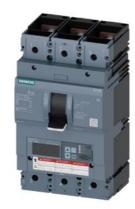
circuit breaker 3VA6 UL frame 600 breaking capacity class C 100kA @ 480 V 3pole, line protection ETU830, LIG, In=600A overload protection Ir=240A ...600A short-circuit protection Ii=1.5...9 x In ground-fault protection Ig=0.2... 1 x In, tg=0.05-0.8s nut keeper kit on both sides
