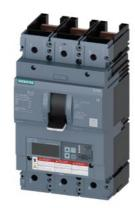
circuit breaker 3VA6 UL frame 600 breaking capacity class C 100kA @ 480V 3-pole, line protection ETU830, LIG, In=600A overload protection Ir=240A...600A short-circuit protection Ii=1.5...9 x In ground-fault protection Ig=0.2...1 x In, tg=0.05-0.8s without connection
