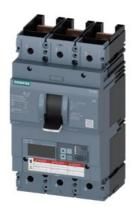
circuit breaker 3VA6 UL frame 600 breaking capacity class H 65kA @ 480V 3-pole, line protection ETU830, LIG, In=600A overload protection Ir=240A...600A short-circuit protection Ii=1.5...9 x In ground-fault protection Ig=0.2...1 x In, tg=0.05-0.8s without connection
