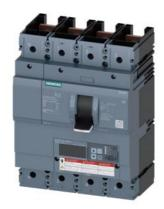
circuit breaker 3VA6 UL frame 600 breaking capacity class H 65kA @ 480V 4-pole, line protection ETU556, LSI, ln=600A overload protection Ir=240A...600A short-circuit protection Isd=0.6..9x In, li=1.5..9x In N conductor protection adjustable (OFF, up to 100%) ground-fault alarm message via EFB300 or COM without connection
