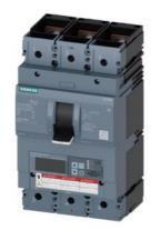
circuit breaker 3VA6 UL frame 600 breaking capacity class H 65kA @ 480 V 3-pole, line protection ETU556, LSI, In=600A overload protection Ir=240A ...600A short-circuit protection Isd=0.6..9x In, Ii=1.5..9x In N conductor protection opt. w. ext. CT; up to 160% ground-fault alarm message via EFB300 or COM nut keeper kit on both sides
