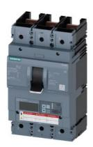
circuit breaker 3VA6 UL frame 600 breaking capacity class H 65kA @ 480V 3-pole, line protection ETU556, LSI, In=600A overload protection Ir=240A...600A short-circuit protection Isd=0.6..9x In, Ii=1.5..9x In N conductor protection optionally with external current transformer, up to 160% ground-fault alarm message via EFB300 or COM without connection
