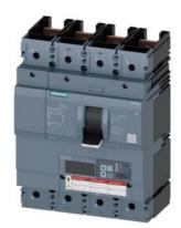
circuit breaker 3VA6 UL frame 600 breaking capacity class H 65kA @ 480V 4-pole, line protection ETU560, LSIG, In=600A overload protection Ir=240A...600A short-circuit protection Isd=0.6..9x In, Ii=1.5..9x In N conductor protection adjustable (OFF, up to 100%) ground-fault protection Ig=0.2...1 x In= tg=0.05-0.8s without connection
