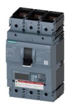
circuit breaker 3VA6 UL frame 600 breaking capacity class H 65kA @ 480 V 3-pole, line protection ETU560, LSIG, In=600A overload protection Ir=240A ...600A short-circuit protection Isd=0.6..9x In, Ii=1.5..9x In N conductor protection opt. w. ext. CT; up to 160% ground-fault protection Ig=0.2... 1 x In, tg=0.05-0.8s nut keeper kit on both sides
