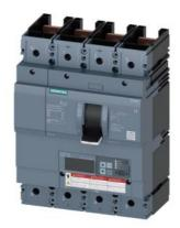
circuit breaker 3VA6 UL frame 600 breaking capacity class H 65kA @ 480V 4-pole, line protection ETU550, LSI, In=600A overload protection Ir=240A...600A short-circuit protection Isd=0.6..9x In, Ii=1.5..9x In N conductor protection adjustable (OFF, up to 100%) without connection
