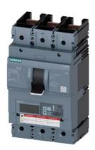
circuit breaker 3VA6 UL frame 600 breaking capacity class H 65kA @ 480V 3-pole, line protection ETU550, LSI, In=600A overload protection Ir=240A...600A short-circuit protection Isd=0.6..9x In, Ii=1.5..9x In N conductor protection optionally with external current transformer, up to 160% without connection
