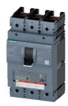
circuit breaker 3VA6 UL frame 600 breaking capacity class H 65kA @ 480V 3-pole, line protection ETU320, LI, In=600A overload protection Ir=240A...600A short-circuit protection Ii=1.5...9 x In without connection
