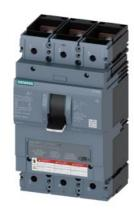
molded case switch 3VA6 UL frame 600 max. sh-circ breaking capacity 100kA @ 480 V 3-pole, line protection MCS110, In=600A without overload protection self-protection Ii=9 x In nut keeper kit on both sides
